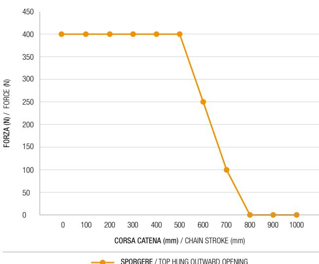
In order to choose the most suitable Comunello Mowin actuator, you have to calculate the necessary FORCE (**F**) to sustain the window movement. Choose the actuator type in accordance with the CALCULATED FORCE (**N**) and the FRAME DIMENSION.
