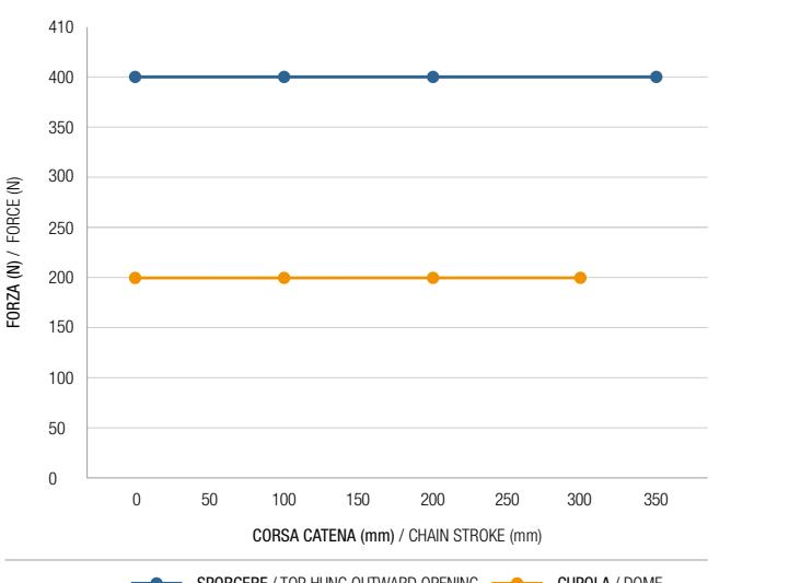
In order to choose the most suitable Comunello Mowin actuator, you have to calculate the necessary FORCE (**F**) to sustain the window movement. Choose the actuator type in accordance with the CALCULATED FORCE (**N**) and the FRAME DIMENSION.
