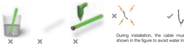
During installation, the cable must be positioned as shown in the figure to avoid water infiltration.
