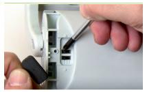
Easily adjustable stroke via dip-switch (up to 9 positions available), also when motor is powered off
