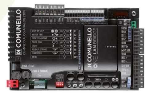
One Dialog Analog control unit 230V which offers the option of local programming as well as managing remote functions and commands via the App directly from a smartphone or tablet. Multilevel menu with the use of only two "Select" and "Set" buttons. An LED-driven system which is easy and intuitive to use.
