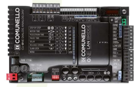
One Dialog Analog 24V control unit which offers the option of local programming as well as managing functions and commands remotely via the App directly from a smartphone or tablet. Multilevel menu with the use of only two "Select" and "Set" buttons. An LED-driven system which is easy and intuitive to use.
