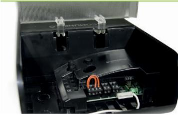
Integrated control unit and receiver. Led function setting and trimmer adjustment for easy programming and diagnosis.
